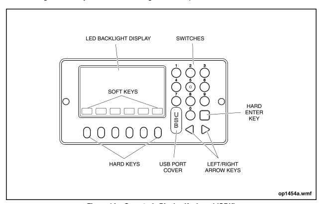
Figure 14: Operator's Display Keyboard (ODK)
