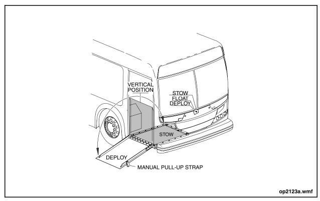
Figure 26: Wheelchair Ramp Operation
