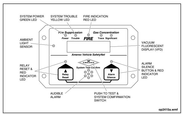
Figure 22: Fire Suppression Control Panel
