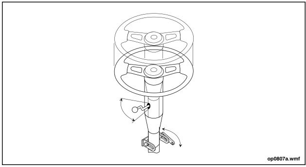
Figure 12: Steering Wheel Adjustment
