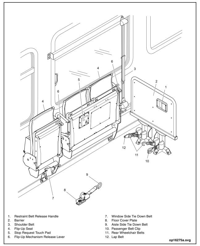
Figure 27: Wheelchair Restraint System (Curbside)
