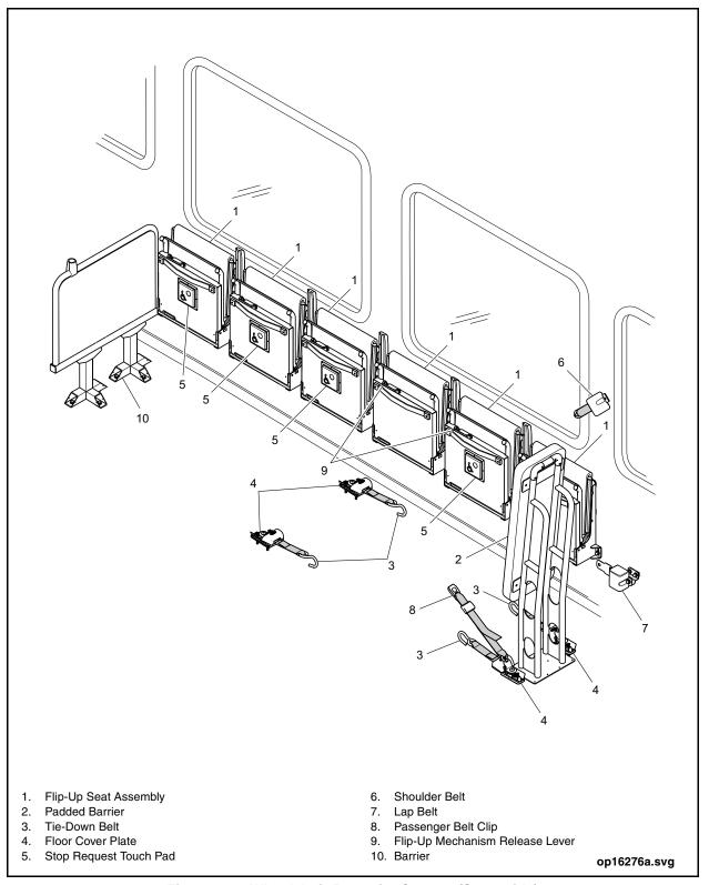
Figure 28: Wheelchair Restraint System (Streetside)
