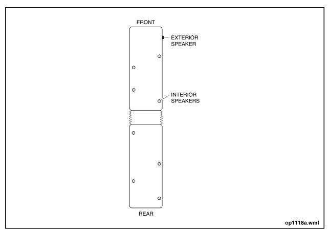
Figure 13: P.A. System Layout
