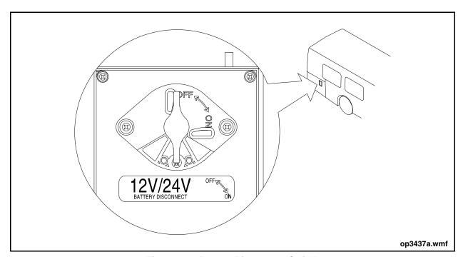
Figure 24: Battery Disconnect Switch
