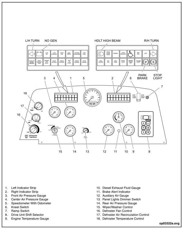
Figure 15: Instrument Panel
