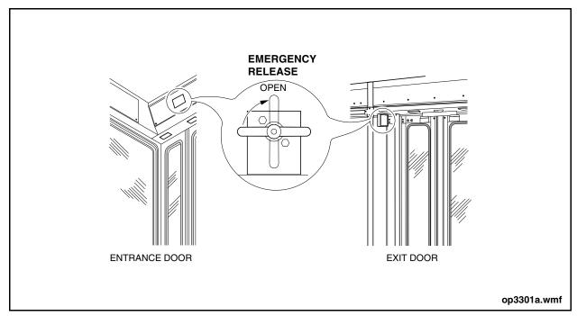
Figure 4: Passenger Door Emergency Release
