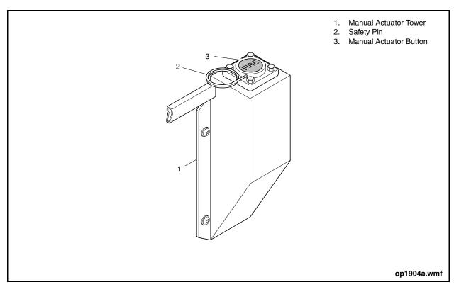
Figure 23: Manual Actuator
