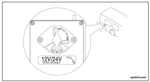
Figure 1: Battery Disconnect Switch
