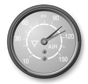
Air pressure must be above 70 psi before air brakes can develop their full effectiveness. The operator should observe the air pressure gauge frequently.
