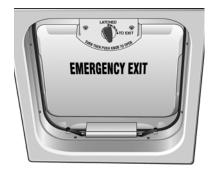
To operate the rear roof hatch:
