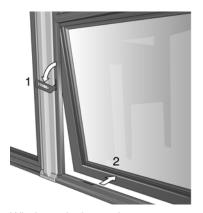
Windows designated as emergency exit passenger windows are hinged at the top and can be pushed out at the bottom for emergency egress.
