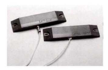
The AT5704 and AT5707 Dynamic Tags are extended-memory, field disturbance, backscatter devices. The memory of the tags can be written to using an asynchronous wire interface. Data written to the tag can then be retrieved remotely by radio frequency from roadside or rail wayside readers.
