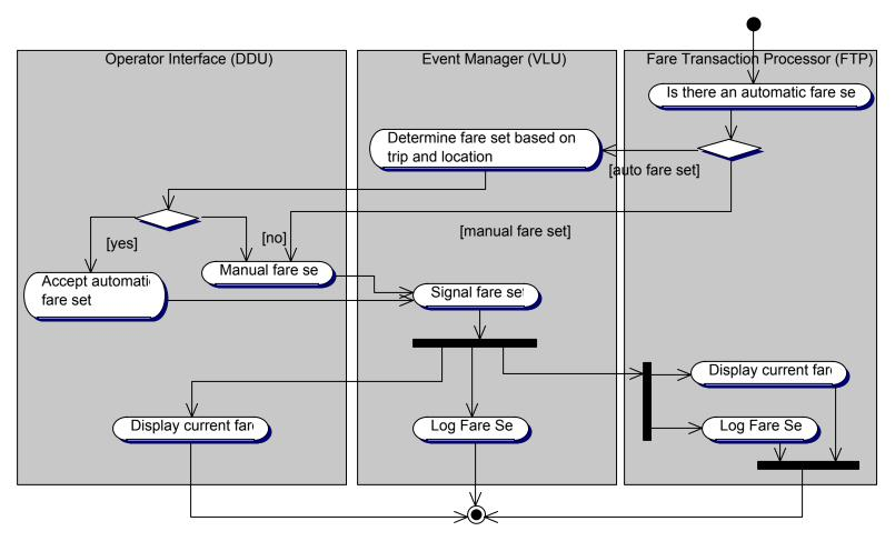
Figure 2.B.4.1.14.RV14.c. Activity Diagram Collect Fare
