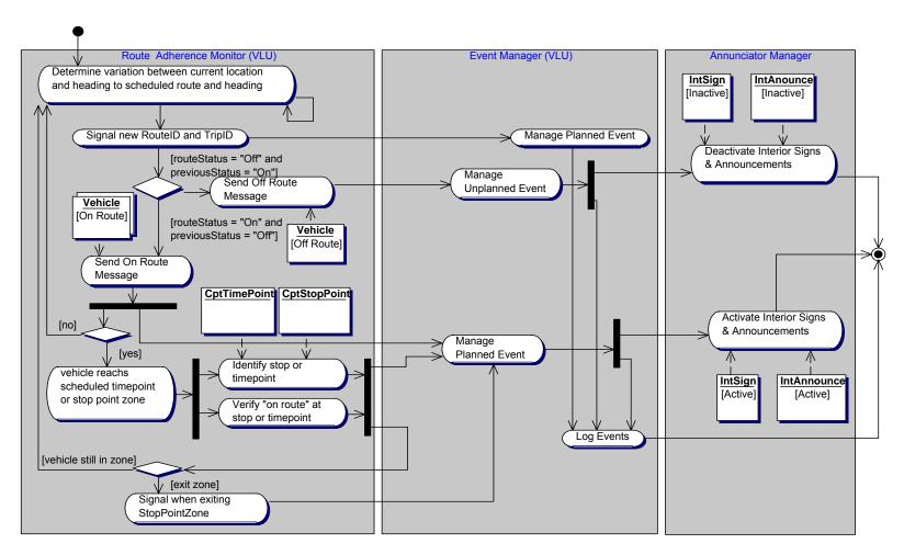
Figure 2.B.4.1.8.RV8.c. Activity Diagram Monitor Schedule Adherence
