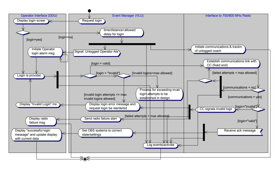
Figure 2.B.2.4.1.1.RV1.e. Activity Diagram Initiate vehicle from warm start
